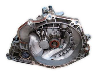
Image 1: When repairing the clutch, inspect the bearing arrangement of the release shaft
